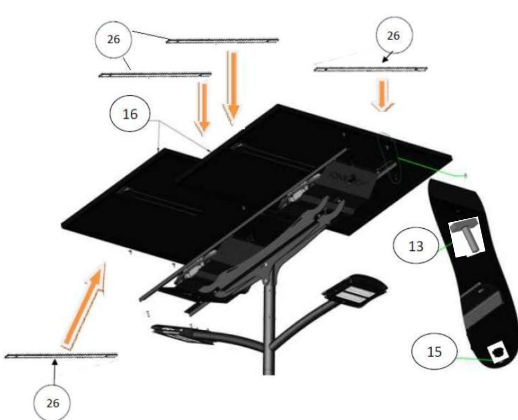
The reinforcement flat n° 26 (optional, only on high wind poles) are to be positioned inside the frame of the PV and to be fixed with screws / nuts 13 and 15.
