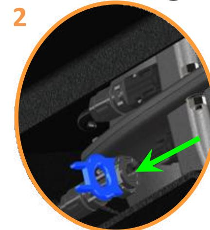
Detach one connector of each PV with the « Universal tool disconnect » n°1.
