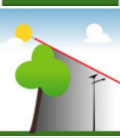
Avoid **any shadow** on the solar panel (trees, houses, traffic signs...). Shadows will considerably impact electricity production of the panel and hence reduce recharging of the battery.
