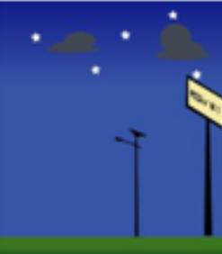
Avoid **artificial light** on the solar panel during nighttime. This could hinder correct detection of sun fall by the panel and can, worst case, completely disable switching on of the light.
