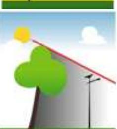
Avoid **any shadow** on the solar panel (trees, houses, traffic signs...). Shadows will considerably impact electricity production of the panel and hence reduce battery charging.
