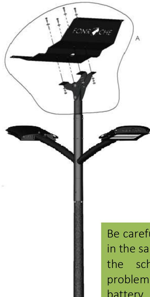
Be careful to set the screws n°8 in the same way as illustrated in the scheme to avoid any problem when installing the battery. Do not forget the washers n°4 and n° 5
