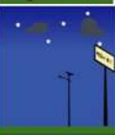
Avoid **artificial light** on the solar panel during nighttime. This could hinder correct detection of dusk by the panel and can, worst case, completely disable light to switch on.
